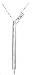
Urethroscope with distal bulb illumination
